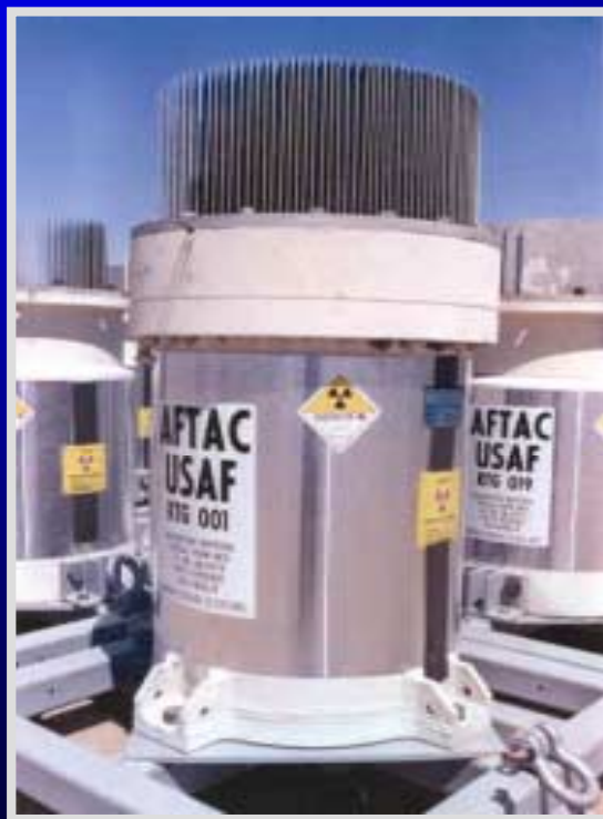
Radioisotope thermoelectric generator (1000 TBq ^{90}\text{Sr} )
